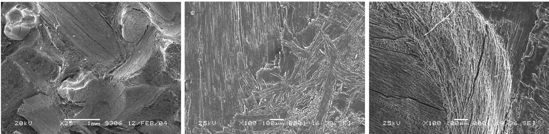
(a) SEM ablation morphology of sample 1# (b1) SEM ablation morphology of sample 2# (b2) SEM ablation morphology of sample 2#
