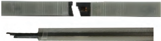
图 17 IM7/CYCOM5320-1 复合材料的 0°压缩破坏模式 Fig. 17 Failure mode in 0° compression test of IM7/CYCOM5320-1 composites
