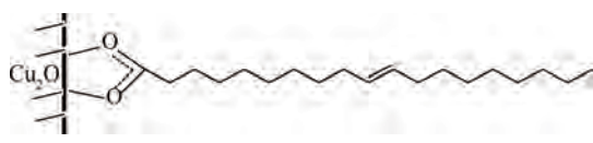
图5 OA中的COO—和Cu原子双齿螯合作用示意图 Fig. 5 Chelating bidentate interaction between COO—group of OA and copper atom
