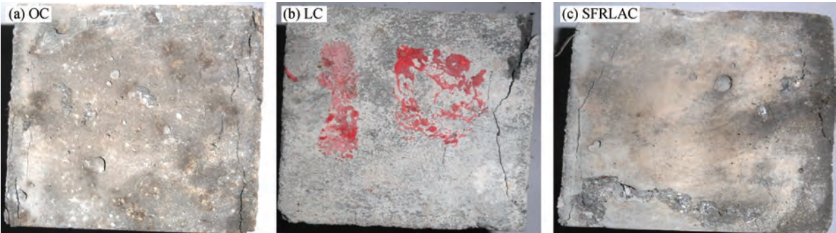
图 3 混凝土试块受压破坏形态 Fig. 3 Failure modes of concrete specimen under compression
