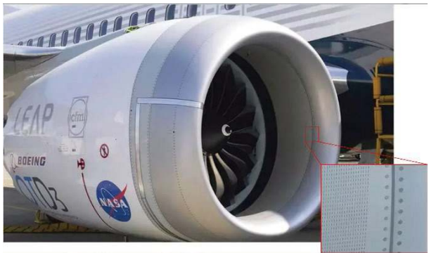
图4 航空发动机短舱声衬 [25] Fig. 4 Acoustic liner for aircraft engine nacelle [25]
