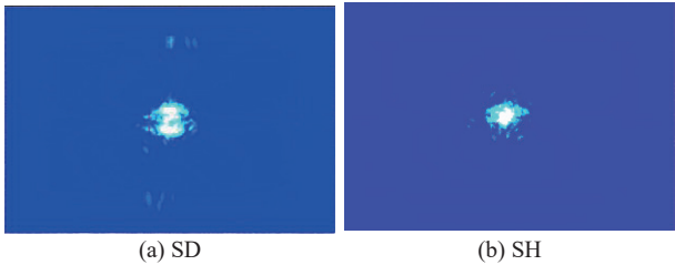
图 8 DE710-T700S 层合板仿真分层损伤累计结果 Fig. 8 Simulated cumulative delamination damage results of DE710-T700S laminate
