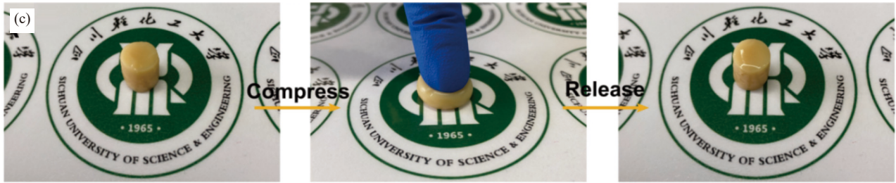
图4 GQDs-TiO 2 /PAM 杂化水凝胶 (1wt%GQDs) 力学性能图片: (a) 交叉和拉伸; (b) 打结和拉伸; (c) 压缩和释放 Fig. 4 Photographs of GQDs-TiO 2 /PAM hybrid hydrogels (1wt%GQDs) under external forces: (a) Cross-bended and stretched; (b) Knotted and stretched; (c) Compressed and released
