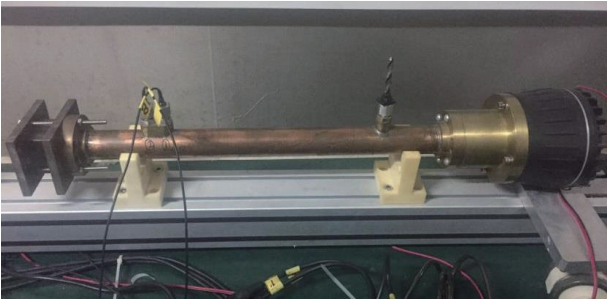
图3 装配测试样品及夹具的阻抗管实物图 Fig.3 Physical drawing of impedance tube for assembling test sample and fixture
