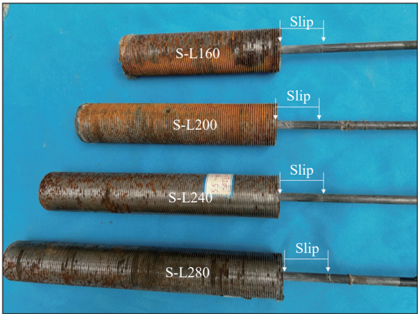
(a) Failure modes of experimental anchorage under static loads
