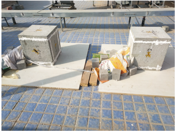
图 8 基准砂浆和 30% 掺量相变微胶囊储能砂浆温控性能试验箱 Fig. 8 Reference mortar temperature control performance test box and the 30% phase change microcapsule energy storage mortar temperature control performance test box
