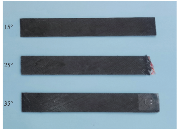
(b) Carbon/glass fiber hybrid ratio 2:6
