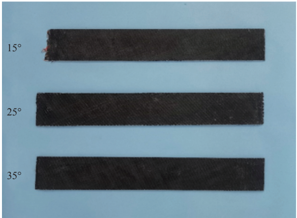
(a) Carbon/glass fiber hybrid ratio 4:4
