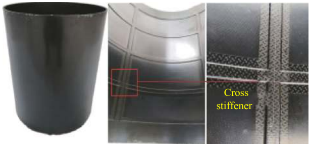
(c) Composite cabin after curing
