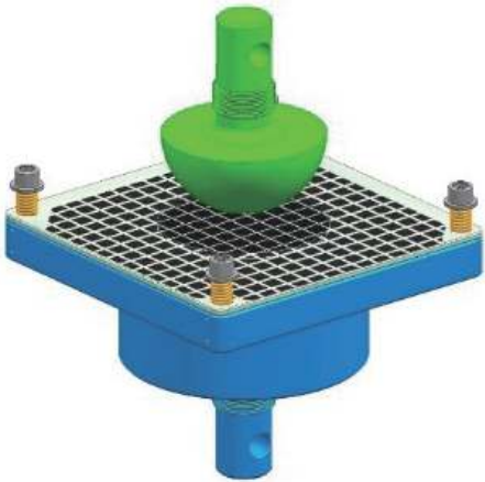
图 9 单层 CF/PC 预浸料的单穹顶结构赋形模型示意图 Fig. 9 Schematic diagram of the preforming model of the single dome structure of CF/PC monolayer prepreg
