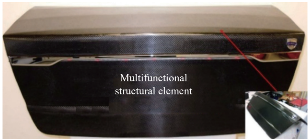
图 12 STORAGE 项目针对沃尔沃车型研发的电动行李箱盖板 [70] Fig. 12 STORAGE project developed an electric luggage cover for Volvo models [70]
