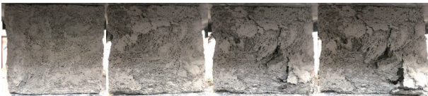
(b) Oblique shear failure
