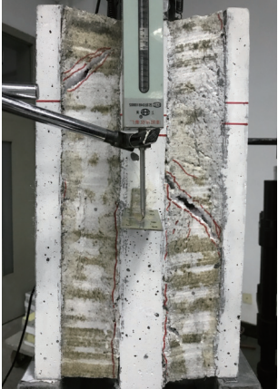
(c) Shear failure of EPS
