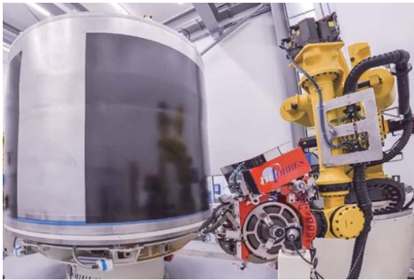
图1 罗-罗公司采用自动纤维铺放 (AFP) 技术制造航空发动机风扇机匣 [6] Fig. 1 Rolls-Royce aero-engine fan casing manufactured by automated fiber placement (AFP) [6]
