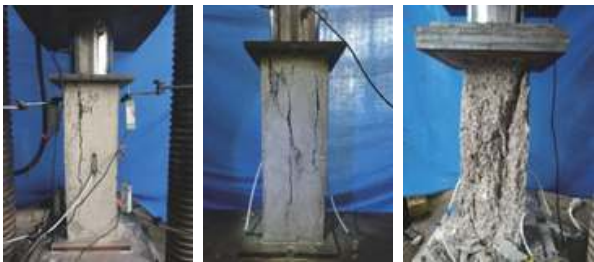
(a) At cracking load (b) At 75% of peak load (c) At peak load
