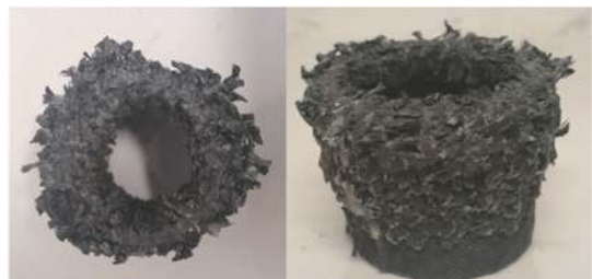
(b) Observation of sample after CF-CF/EP compression
