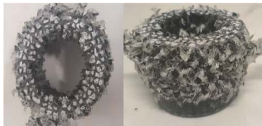
(b) Observation of sample after CF-GF/EP compression
