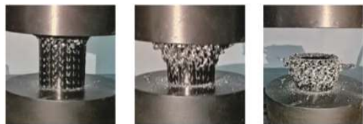
(a) CF-GF/EP axial compression process diagram
