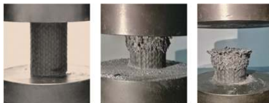
(a) CF-CF/EP axial compression process diagram
