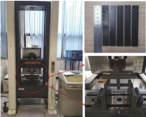
图 10 衬经 2.5D 机织引纱加纱复合材料三点弯曲测试 Fig. 10 Three-point bending test 2.5D woven with warp-stuffer containing pull-out and add-in yarn composites
