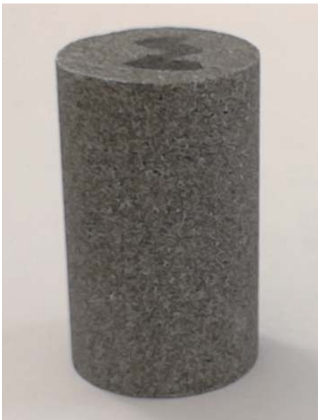
图3 FAC/Al 基复合泡沫试样 Fig. 3 Sample of FAC/Al syntactic foam
