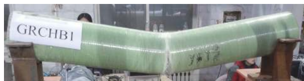
(a) Failure diagram of flexural member
