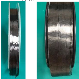
(a) Carbon fiber (CF) after wide-spreading
