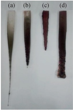
图 5 n\text{Mg}(\text{OH})_2 60/\text{EVA} 、MRP60/EVA 和 n\text{Mg}(\text{OH})_2 50\text{-MRP}10/\text{EVA} 复合材料垂直燃烧实验后残余物的数码照片 Fig. 5 Digital photos of residue of n\text{Mg}(\text{OH})_2 60/\text{EVA} , MRP60/EVA and n\text{Mg}(\text{OH})_2 50\text{-MRP}10/\text{EVA} composite after vertical burning test (a) pure EVA; (b) n\text{Mg}(\text{OH})_2 60/\text{EVA} ; (c) MRP60/EVA, (d) n\text{Mg}(\text{OH})_2 50\text{-MRP}10/\text{EVA}
