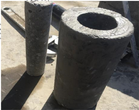
图 2 SF/NC 空心圆柱试件制备 Fig.2 Preparation of SF/NC hollow cylinder specimens
