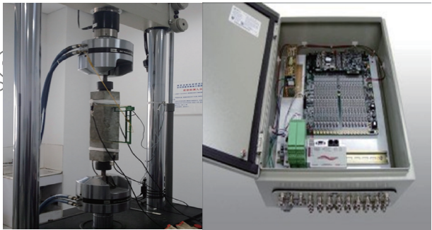
图 1 混凝土循环拉伸声发射特性试验系统 Fig. 1 Acoustic emission characteristic test system of cyclic tension of concrete
