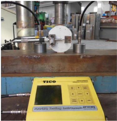
图 5 超声波速法检测混凝土裂缝 Fig. 5 Detecting concrete cracks based on changes of ultrasonic velocity
