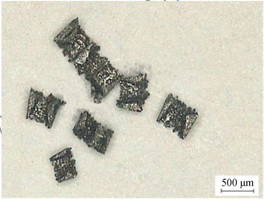
图 11 PCD 刀具切削 SiC p /Al 复合材料的切屑形态 Fig. 11 Morphology of chips in cutting SiC p /Al composite using PCD tool
