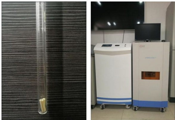
图2 丁羟包覆层的核磁测试样品和设备 Fig. 2 Specimen and equipment of NMR test for hydroxyl-terminated polybutadiene inhibitor
