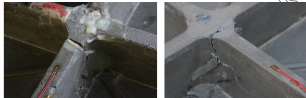
(a) Cracks of the stiffened bar (b) Crack trend of the propagation
